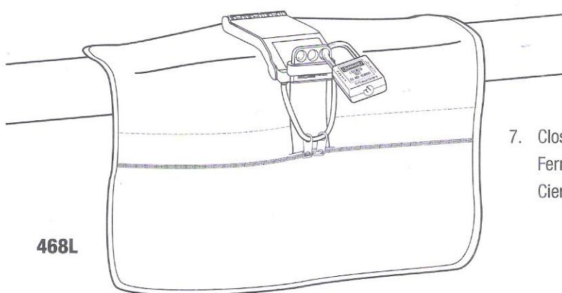
7. Close locking mechanism and apply padlock
