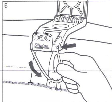
6. Thread zipper tie through both zipper tabs and place end in pocket in locking mechanism.
