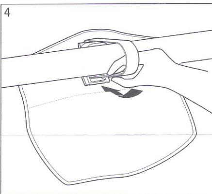
4. Apply device on valve and wrap strap around valve.
