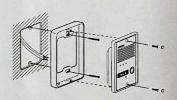
After attaching the body supporter with 2screws, put the indoorstation into the grooves of body supporter, and then fix it with screws.
