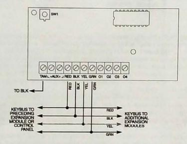
**TAM** - This can be used to tamper the cabinet in which the PC5208/4 is mounted. Connect a normally closed (NC) switch across TAM and BLK. If the tamper is not being used connect a piece of wire across TAM and BLK to remove the trouble condition.
