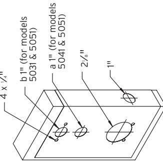
**A-2** For Models 5041 & 5051 only. When installing Model 5021, skip to step A-4.
