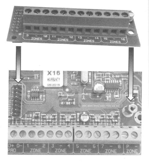
The IDS Plug-in Zone Expander connects directly onto the X64 Alarm Panel via connectors, as shown in the diagram above. The Plug-in Zone Expander is permanently allocated to zones 9-16. This cannot be changed.
